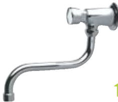
TE 53 Temporized (timer) frontal mounted, with "S" spout, 1/2" tap, all in c.p. brass, opening time 6-8 seconds.
