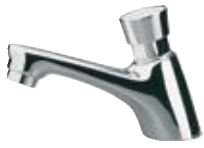
TE 15 Temporized (timer) pillar tap, 1/2", all in c.p. brass, opening time 6-8 seconds.
