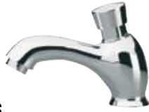
TE 16 Temporized (timer) pillar tap, 1/2", all in c.p. brass, opening time 6-8 seconds.
