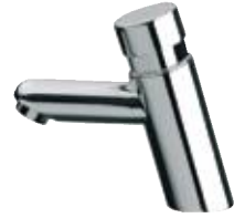
TE 18 Temporized (timer) pillar tap, 1/2", Minimal, all in c.p. brass, opening time 6-8 seconds.
